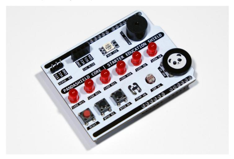
In addition to these components, our shield also includes connections for a mini servo and I2C OLED display that provide even more opportunities for experimenting. The mini servo can be used to control small motors and create moving parts in your projects, while the I2C OLED display allows you to display text and graphics for a more interactive experience.
