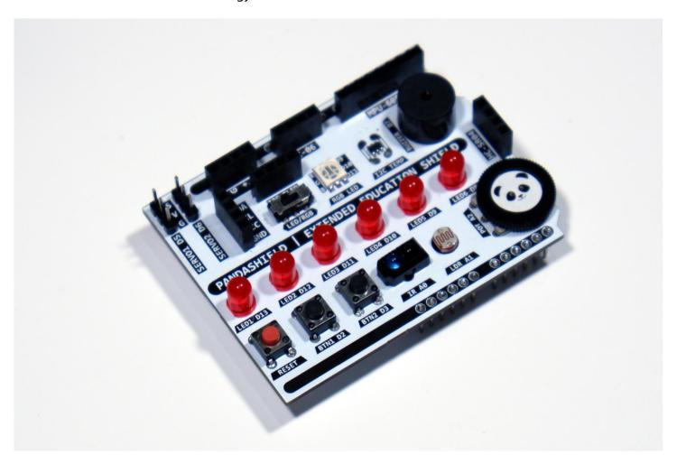
In addition, the shield includes an external universal sensor connection, compatible with various KY type Arduino sensors. This ensures compatibility with a wide range of sensors and expands the versatility of the PandaShield even further.
