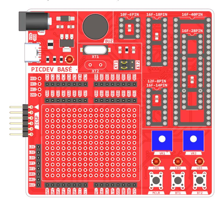
**METE HOCA PICDEV BASE** combines lots of different components in a small package. It has six different PIC microcontroller series support, three LEDs, three buttons, two potantiometers, a passive buzzer, an onboard 4 MHz crystal oscillator, USB Type-C, barrell jack, ON LED and 5 Volt power regulator.
